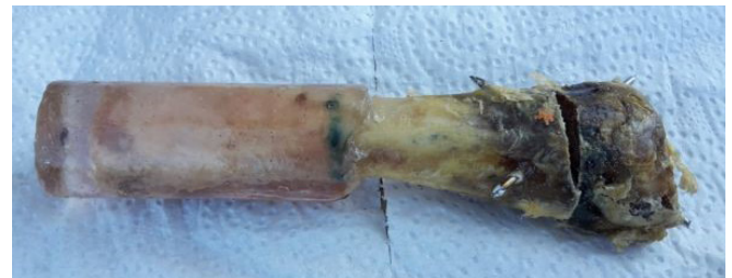
Figure 1. Polyester embedded, ready to test material.
